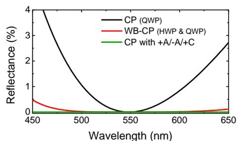
**Figure 5.** Reflection spectra of the CP, WB-CP, and CP with +A/-A/+C plates for normal incidence.
