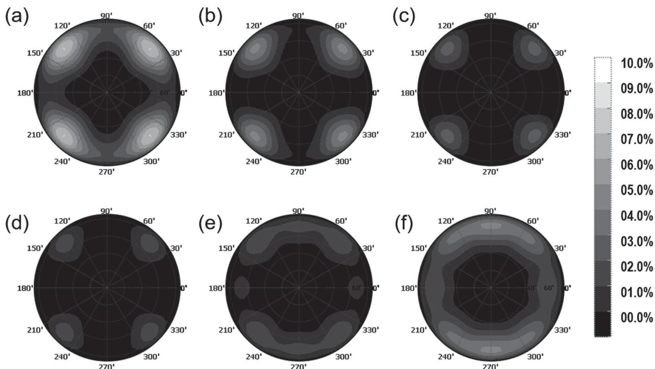
**Figure 4.** Calculated iso-luminance contours with the  $\Delta nd$  of the positive C plate as a parameter: (a) 0; (b) 20; (c) 40; (d) 60; (e) 80; and (f) 100 nm.
