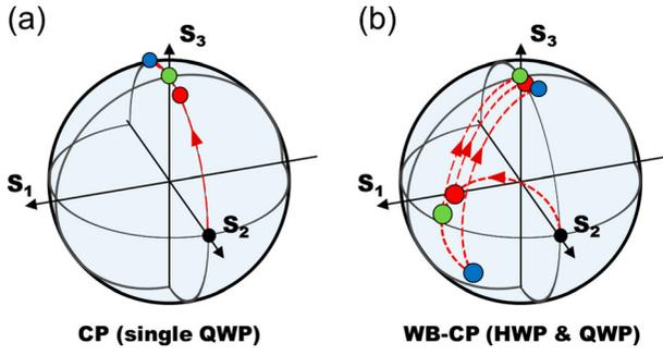
**Figure 1.** Polarization change on the Poincaré sphere of each color (450, 550, and 650 nm wavelengths) by the (a) CP and (b) WB-CP structures for normal incidence.
