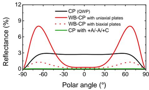
**Figure 6.** Reflectance of the CP, WB-CP, and CP with +A/−A/+C plates vs. the polar angle at the 0° azimuth angle.
