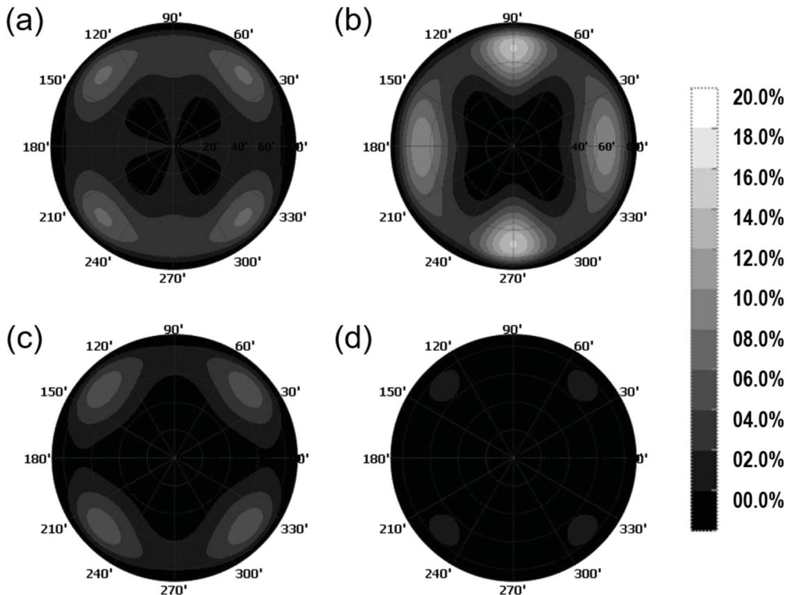
**Figure 7.** Calculated iso-luminance contours of the (a) CP, (b) WB-CP with uniaxial plates, (c) WB-CP with biaxial plates, and (d) CP with +A/−A/+C plates.
