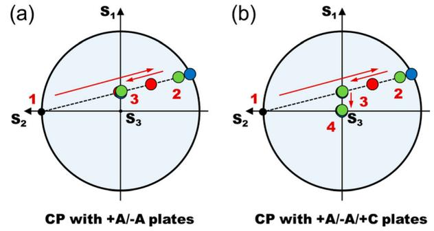
**Figure 3.** Polarization states of each color (450, 550, and 650 nm wavelengths) in the CPs with (a) +A/−A and (b) +A/−A/+C plates on the  $S_1$ – $S_2$  plane of the Poincaré sphere under oblique incidence ( $\theta = 70^\circ$ ,  $\varphi = 0^\circ$ ).
