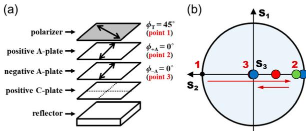
**Figure 2.** (a) Compensation scheme of the CP with +A/−A/+C plates. (b) Polarization change of each color (450, 550, and 650 nm wavelengths) on the Poincaré sphere for normal incidence.
